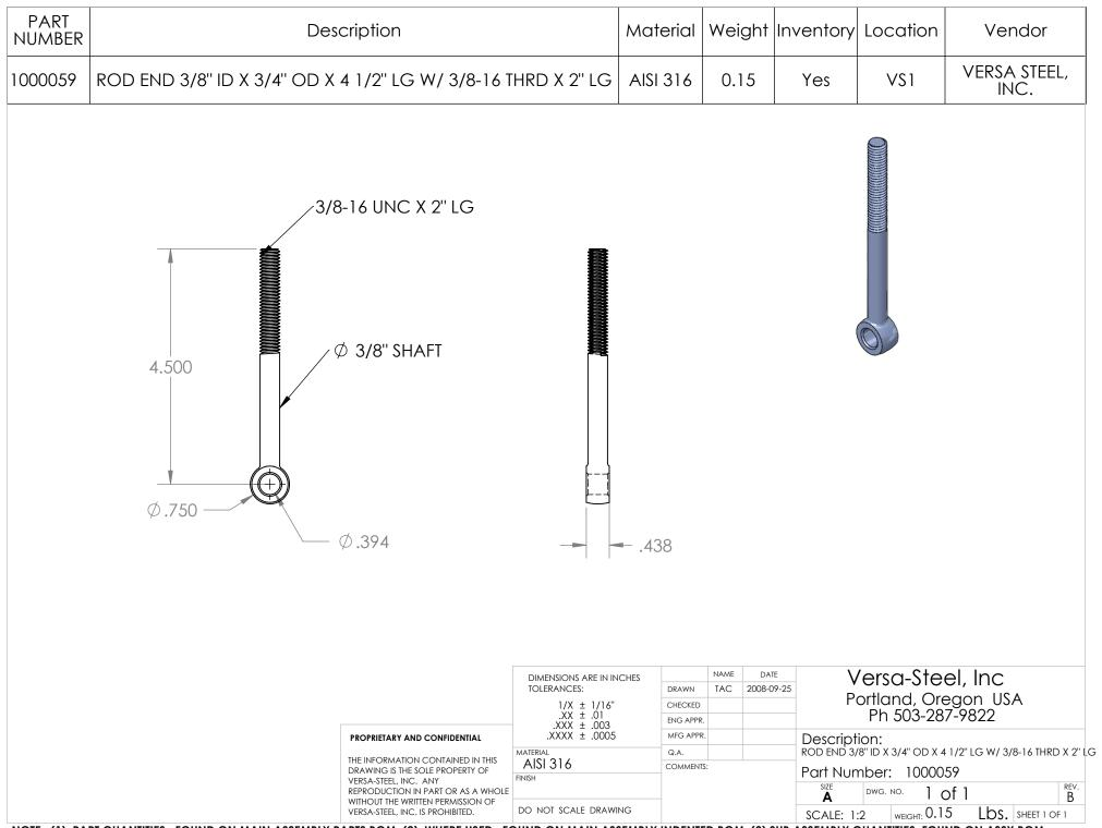
NOTE: (1) PART QUANTITIES: FOUND ON MAIN ASSEMBLY PARTS BOM (2) WHERE USED: FOUND ON MAIN ASSEMBLY INDENTED BOM (3) SUB ASSEMBLY QUANTITIES: FOUND ON ASSY BOM
